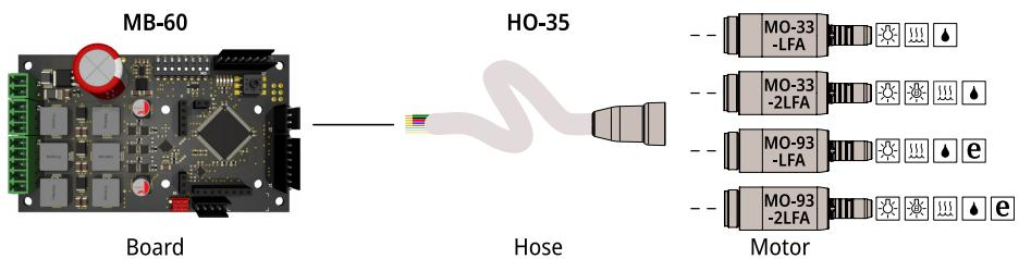
The **S-60** medical device, composed of a micromotor (prefix **MO**), an electronic board (prefix **MB**) and a hose connection (prefix **HO**), is intended to drive a straight or contra-angle handpiece as part of a dental treatment unit.
